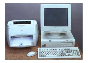
The Administrative Workstation includes color monitor, keyboard, mouse, printer, software, CD/RW, and WAN connection to provide for real-time feature administration, report generation, and monitoring and recording access. Speakers are provided for recording playback and live call monitoring.
