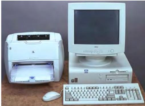
The Administrative Workstation includes color monitor, keyboard, mouse, printer, software, CD/RW, and WAN connection to provide for real-time feature administration, report generation, and monitoring and recording access. Speakers are provided for recording playback and live call monitoring.
